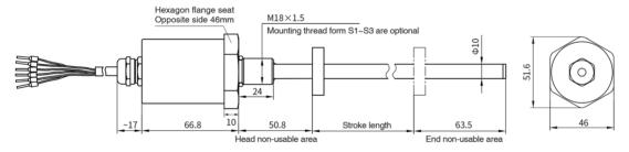
Note: It is equipped with standard Magnet ring kit 288501, with magnetic isolation gasket and fixing screw.
