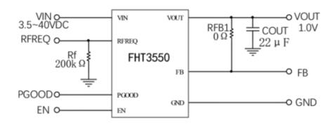
Typical Application Circuit for 1.8V Output
