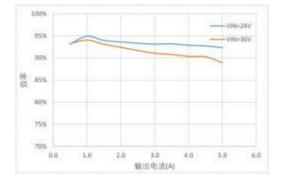
Output Current vs Efficiency (Vout=3.3V)
