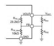
Fig. 1 Voltage divider resistor for setting output voltage
