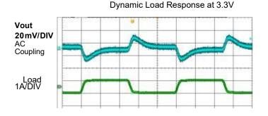
40 us/DIV Vin=12V , Vout=3.3V,lout=3A-4A , 1A/us Output Capacitance=4\*22uF+0.1uFCeramic Capacitor
