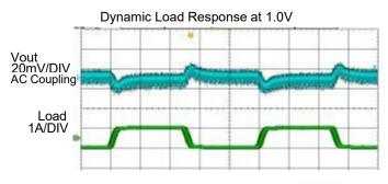
Vin =12V, Vout=1.0V, lout=3A-4A, 1A/us Output Capacitance=4\*22uF+0.1uFCeramic Capacitor
