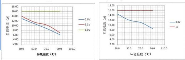
12Vin Derating Curve for Ambient Temperature with 4 Channels in Parallel Configuration 5Vin Derating Curve for Ambient Temperature with 4 Channels in Parallel
