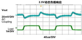
Vin=12V, Vout=2.5V, lout=3A-4A, 1A/us Output Capacitance=4\*22uF+0.1uFCeramic Capacitor
