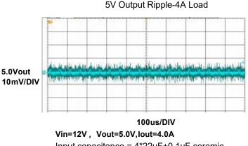
Input capacitance = 4\*22uF+0.1uF ceramic capacitor Output capacitance = 4\*22uF+0.1uFceramic capacitor 20MHZ bandwidth limitation
