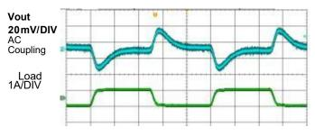
40 us/DIV Vin=12V , Vout=3.3V,Iout=3A-4A , 1A/us Output Capacitance=4\*22uF+0.1uFCeramic Capacitor
