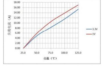
5Vin Derating Curve for Case Temperature with 4 Channels in Parallel
